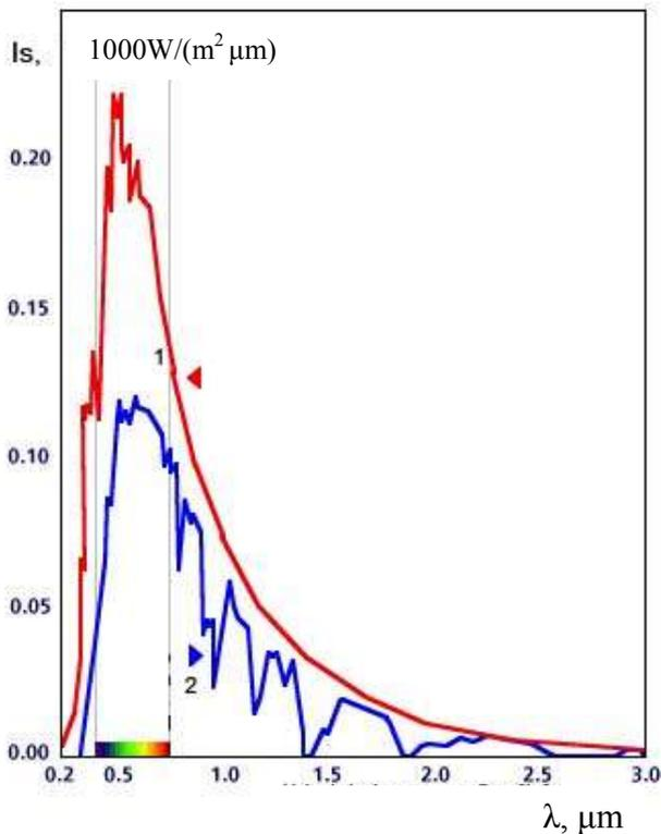
Fig. 2.1. Spectral irradiance of solar light at the upper border of Earth atmosphere (1) and near Earth surface [2]. The peaks on solar spectrum near Earth surface correspond to absorption lines of  $\text{H}_2\text{O}$ ,  $\text{CO}_2$ ,  $\text{O}_3$  atmospheric gases
