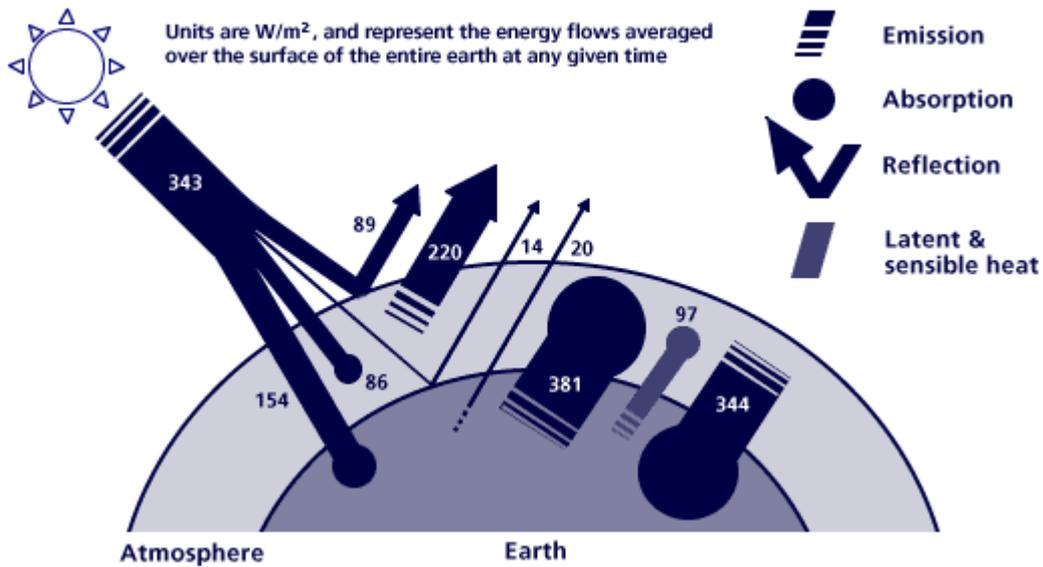
Fig. 2.2. Solar radiation energy flows are averaged over total area of Earth at any time and are measured in  $W/m^2$
