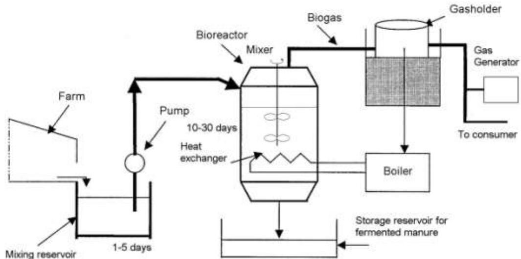
Fig. 7.4. The technological scheme of biogas production
