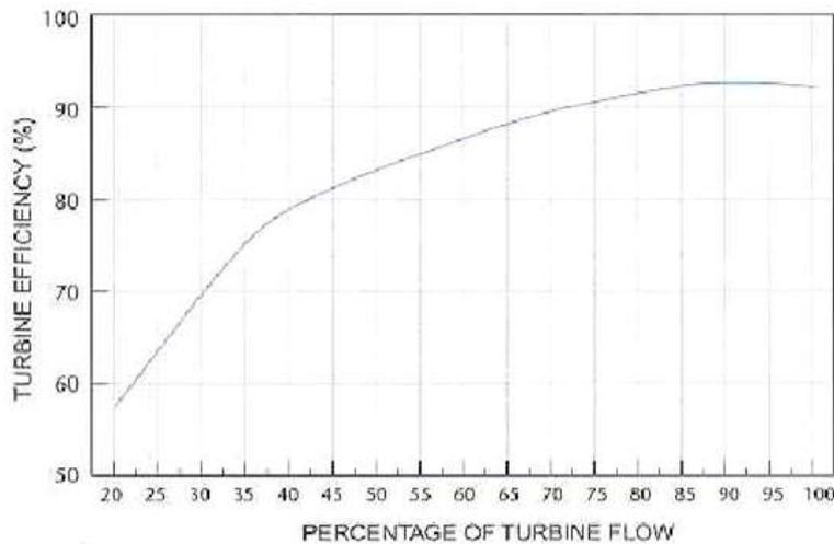
Fig. 10.5. Francis type turbine efficiency curve
