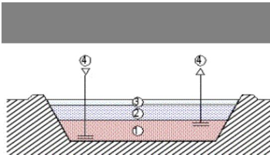
Fig. 4.5. Solar pond: 1 – water layer with high concentration of salt, 2 - water layer with intermediate concentration of salt, 3 - water layer with low concentration of salt, 4 – input of cold water and discharge of warm water.
