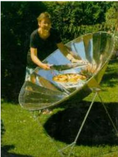
Fig. 3.7b. Parabolic dish solar cooker
