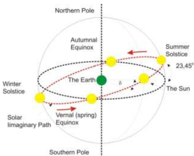
Fig. 2.4. Solar movement on imaginary celestial sphere. Vernal equinox on March 21, autumnal equinox on September 23,  $\delta$  – declination of the sun` sun angular position in respect to celestial equator at noon.  $\delta_0 = 23^{\circ}27' = 23,45^{\circ}$
