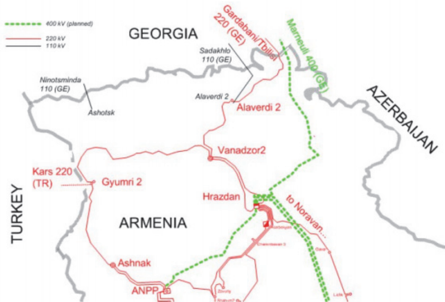
Fig 4. Armenia electricity transmission network 8
